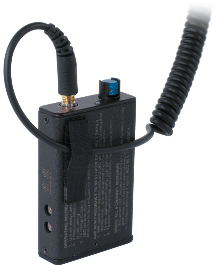
Figure 2 - Headphone cord strain relief
